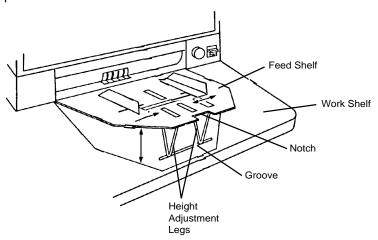
To automatically feed multiple documents, the feed shelf should be in the raised position (as shown above). To raise the feed shelf, grasp the notch and lift the feed shelf. Swing the height adjustment legs out and insert them into the groove on the work shelf.
